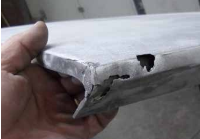
Figure 5. Top: A small amount of rust damage was found on the trailing edge of the passenger door. Bottom: Repairs were made by welding in patches and grinding it smooth.
